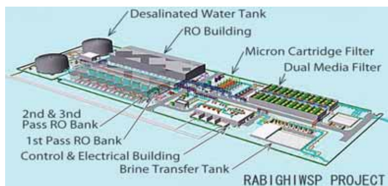
Figure 28: Plant schematic for a Mitsubishi-designed RO plant 14
